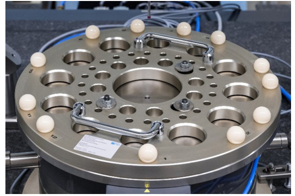
Ball plate for the reduced three-rosette method with 12 irregularly arranged balls
