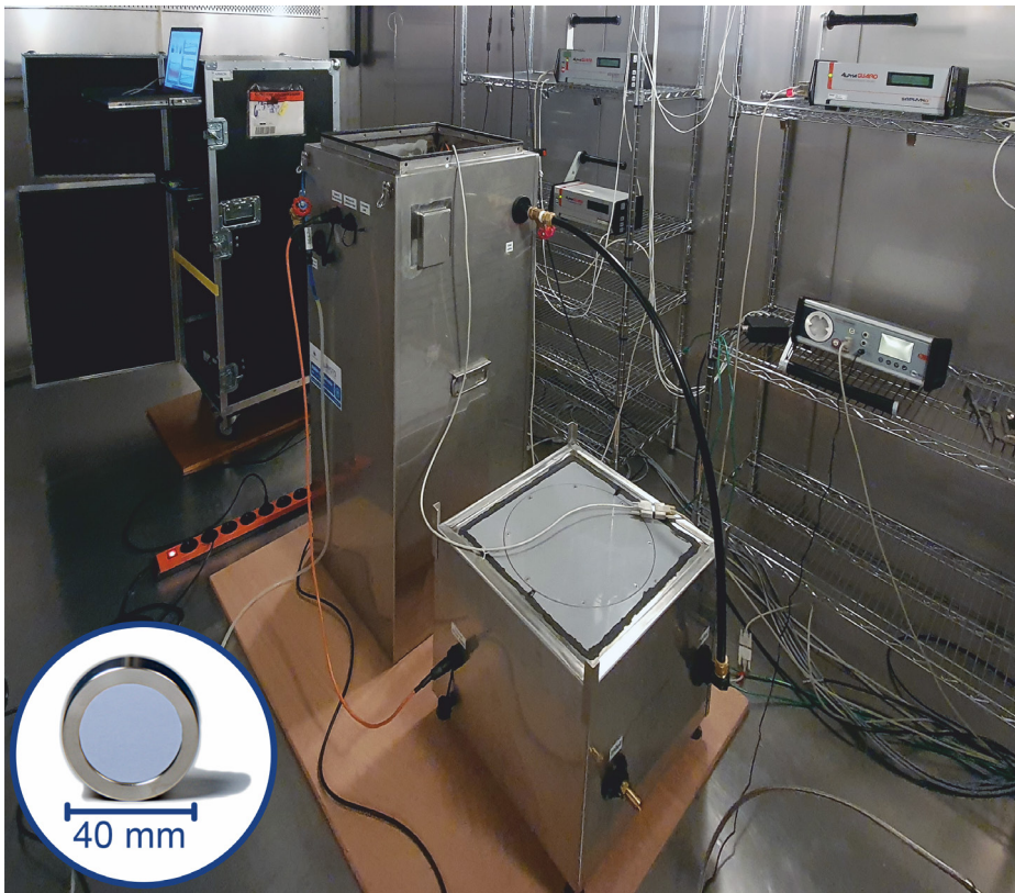
The new transfer standards for outdoor air radon activity concentrations: ANSTO 200 L in the foreground (on the wooden plate) and ARMON v2 in the background (black transport box) in PTB's climate chamber. Inset: the new Integrated Radon Source/Detector (IRSD)
